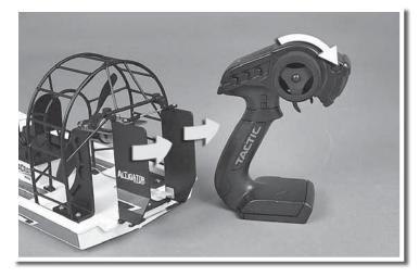
Check the steering direction to make sure when the wheel is turned right or left the twin rudders correspond in the proper direction.
